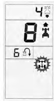
Foraksel tilkoblet premanent ( symbolet for forakslen blinker )
