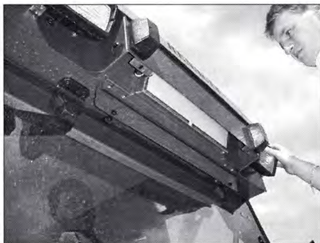
LUFTFILTER I CERGOS KABINE
