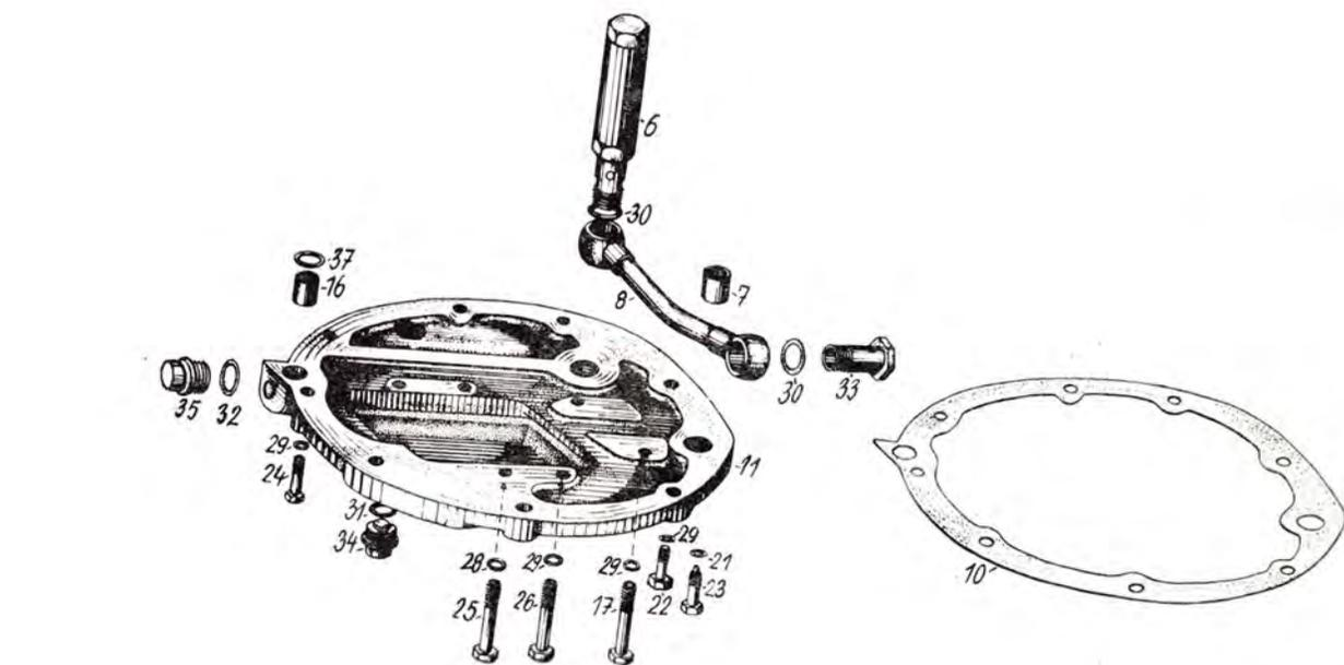
**+ ČERPADLO HYDRAULIKY**
